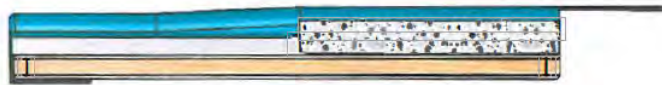
(Fig 2): Side Cross Section shows position of foam inside the sleeve (front flap open).
