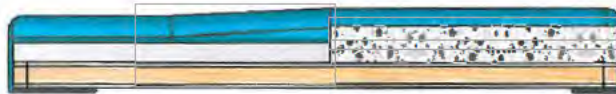
(Fig 5): Side Cross Section shows position of foam inside the sleeve (front flap closed).
