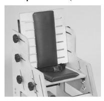
Note: The padded back has already been attached. The padded seat pad attaches to the seat with hook and loop fastener. Remove the (1) self-adhering strip of loop fastener from the pad. Adhere the loop fastener to the top of the seat. Position the pad on the seat and secure the hook and loop fastener.
