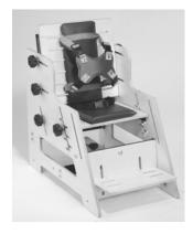
Note: The butterfly harness should be positioned on the chair so that the top of the butterfly straps are even with the shoulders and the buckle is below the collarbone. Adjust the length of the top straps to position the chest piece at the desired location on the chest (see below). Provide a "snug" fit by pulling on the lower set of straps only.
