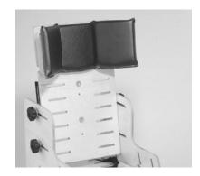
**B.** Attach the wedges to the front of the headrest. Place the knobs with bolts through the desired slot on the backside of the headrest. Secure in the pre-installed T-nuts on the support wedge. Place a washer between the knob and the wood. **Tighten securely.**
