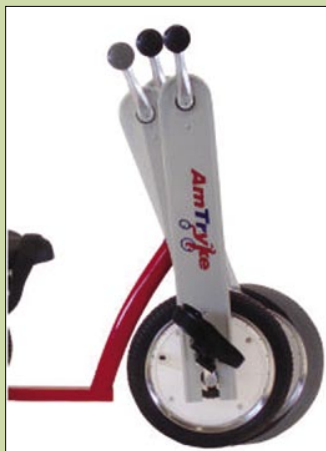
Hinged Front End with Three Positions
