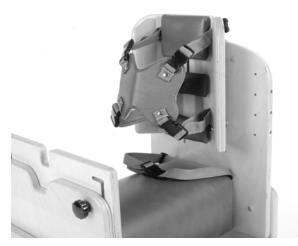
Attach the wooden "yoke" to the back of the chair. This can be placed on the "inside" or the "outside" of the chair back depending on the depth of the seat needed. Place the (2) hex bolts through the pre-drilled holes. Place a nylon washer between the wood and the knob. Secure with small knobs. Tighten securely. Note: For smaller users DO NOT attach the "yoke".
