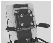
The Butterfly attaches to the chair with straps secured around the back pad. It should be adjusted such that the top of the strap is level with the shoulders. To do this: loosen (or remove) the back pad from the back of the chair by loosening (or removing) the (2) Phillips head screws on the backside of the chair. Slide the straps to the desired location on the pad and tighten (or replace) the Phillips head screws.
