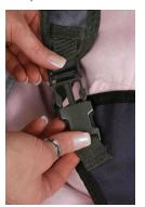
Push down on the silver center button located between the passengers knees and pull the webbing out to the end.
