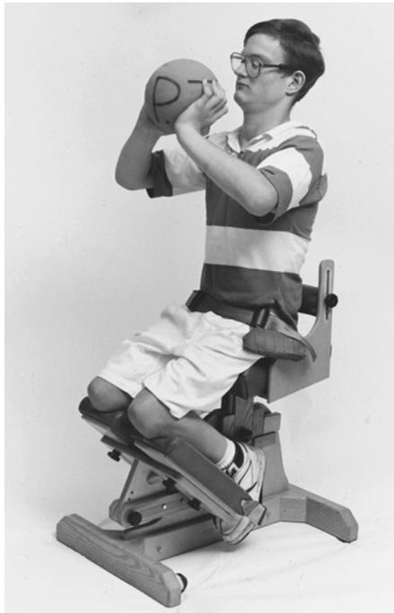
4. **Adjust the kneel pads.** The pads slide “vertically” in the slots on the base when the (4) knobs are loosened. The kneel pad assembly moves up and down on the curved center piece, and the pads can be angled by positioning the bolt through one of the four holes in the underneath gusset. **Note:** The support bar that attaches the kneel pad assembly to the contoured centerpiece is slotted to adjust the depth of the assembly. **Tighten all knobs securely before use.**
