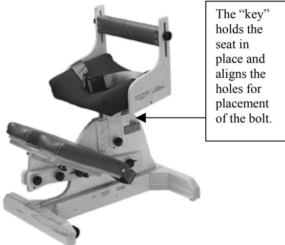
1. **Adjust the seat height.** The seat assembly adjusts to three heights. Insert either end of the wooden "key" (found in the holder at the back of the base) into the seat stem for the two top holes, or lower the seat all the way for the lowest setting (and store the "key" in the holder). The key lines up the respective holes so the bolt can be easily inserted. Place a nylon washer on the bolt and secure with a knob with threaded insert. **Tighten securely.**
